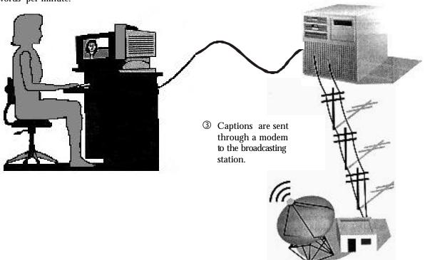
4 Captions are encoded onto line 21 of the television signal and broadcast along with the program.
